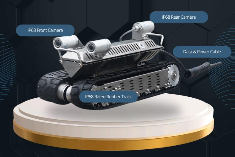
The ProInspect is a durable, adaptable solution for inspecting and maintaining pipelines, sewers, and underground systems. With IP68 waterproofing, advanced speed control, and customisable features, it delivers reliable performance across industries such as oil & gas, water management, and utilities.
