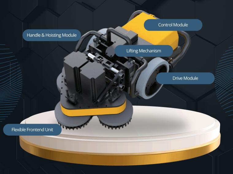
The FlexPrep ensures precise surface preparation for industries such as oil & gas, marine, and infrastructure, improving coating adhesion and corrosion protection. Its adjustable roughening strength, automated lane change, and route planning enhance efficiency, providing a reliable solution for long-lasting asset maintenance.
